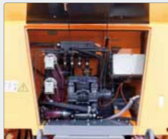
All vital components located together in an enclosed machine house, which offers protection against salt dust. Furthermore, the design has focus on increased user friendliness for drivers and service staff.
